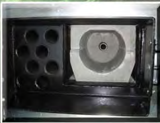
FRONT VIEW OF REACTION CHAMBER SECONDARY AIR EXTRA HEAVY DUTY REACTION OFFSET CHAMBER NOZZLE FOR OPTIMAL TURBULENCE
