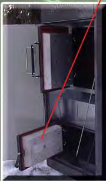
HEAVY DUTY REACTION CHAMBER DOOR WITH INSPECTION GLASS
